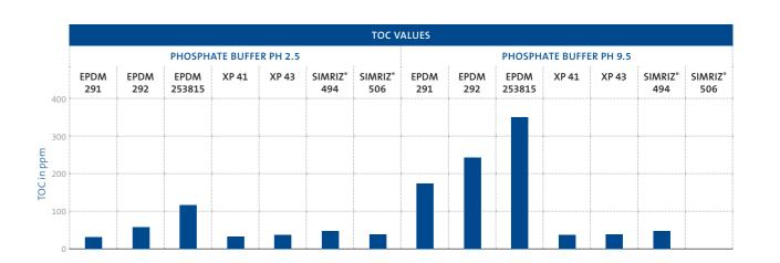
By means of the Extractables-study it could be found out that the tested materials of Freudenberg show a very slight extract value. The extractable portion of EPDM-compounds was under 3%. With the fluorous materials the portion was under the detection limit. Additionally the TOC-results prove the purity of the tested materials.
