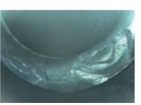
**Grease swelling** – EPDM swells in mineral oil and mineral fat and becomes softer. The damage is evident in shell-like disruptions with relatively round edges. Even individual pieces can break off. It is necessary to check whether the correct assembly grease was used. Generally, EPDM may only be lubricated with silicone grease. In addition, the product-specific information, such as fat concentration, temperature etc., should be recorded in order to verify the possibility of using EPDM.
