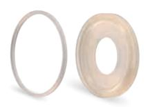
VMQ silicone rubbers are highly polymeric vinyl-methylpolysiloxanes. Silicone is quite widespread as a material in butterfly valve seals. Due to its low volumetric expansion under the influence of media and its high elasticity, the butterfly valve switches reliably until the end of its service
